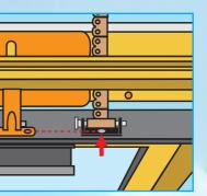
Once the chain is fully extended, use the connector bar to attach the chain to the vent flap bracket. Ensuring that you keep the chain straight, line up the vent flap bracket as shown (fig 8) and mark.
