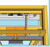
In order to attach the sash to the motor, fully extend the chain connector by pressing the downarrow button on the wall mounted switch (fig 7). If you have opted not to fit a wall mounted switch you will then have to activate it using your remote control.
