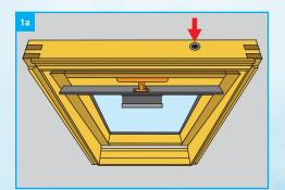
If the interior ceiling is not finished, the cable can be passed through the pre-drilled hole by removing the thimble (fig 1a).
