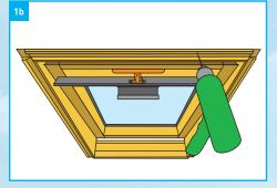
If the ceiling is finished a 10mm hole must be drilled through the top of the frame (figs 1b, 1c & 1d), 20mm down from top and 145mm in from the side of the frame.
